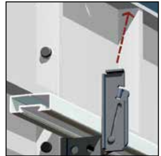
~Removal of waler board~
